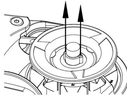
4. Remove the two Drive Pins from the key ways on either side of the Main Shaft.
