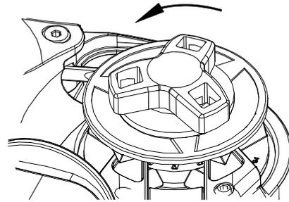
2. Undo the Clutch Nut using 1/2 inch ratchet and or the Pro-Series winch handle & unscrew by hand. **Note You can only use the Pro-fish upgrade kit if there is a threaded hole in the end of the shaft.**
