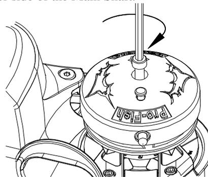
6. Place the Brass Washer onto the Cap Screw. Put Loctite (provided) onto thread of bolt and fit into the end of the Main Shaft. Tighten up using allen key provided (21Nm, 15.4 lbf/ft) . Allow at least **15mins** for Loctite to cure before use.
