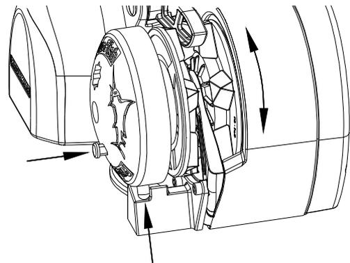
10. Check the 'freefall' feature by loosening the Pro-fish Cap & spinning the Gypsy with your hands. The Gypsy should be able to spin freely.
