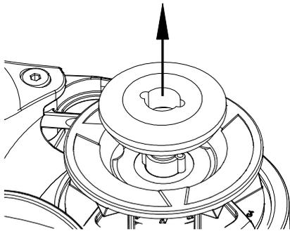
3. Remove the Gypsy Cone from the Main Shaft.
