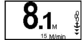
Settings and measurements are saved if the unit is turned off or the battery fails. Counting continues if the windlass is operated by another control eg foot switches.
