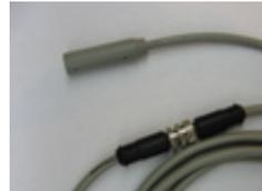
A 2m male/female cable (Part #9505) plus a gender changer (Part #9510) will be required to connect the extension cable to the base station.
