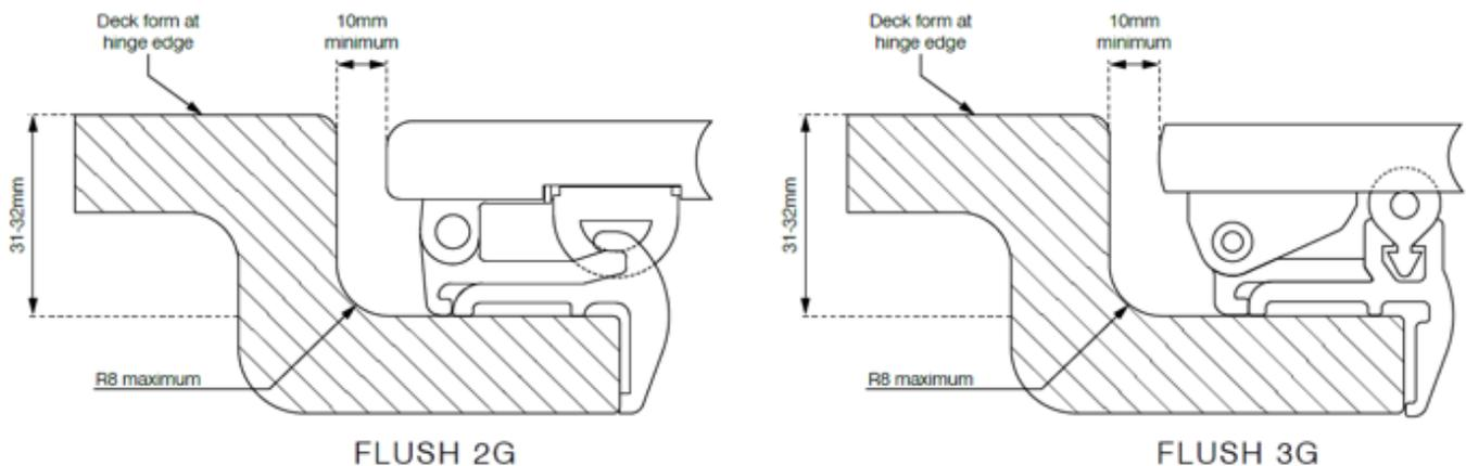
*It is essential that the lower frame is placed square on the deck opening. The operation of the hatch should be checked before sealing and fastening to the deck. Each installation should allow for either drainage channels or tube around the hatch to ensure no excess water can become trapped.*
