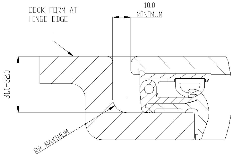
***It is essential that the lower frame is placed square on the deck opening. The operation of the hatch should be checked before sealing and fastening to the deck***
