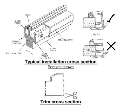
Adjust the trim moulding to the calculated length H by cutting the inner edge only to suit, using a fine toothed saw or tin snips, such that when fitted the trim clips to the inner frame. Snap the trim moulding into final position making sure that it clips onto the inner frame and is fully home all around its perimeter. It is a simple matter to remove the trim by prising it away on the outside edge, refit by snapping back onto the inner frame.
