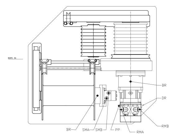
NDTE: RMB CONNECTED TO PORT A RMA CONNECTED TO PORT B PP CONNECTED TO PORT X5
