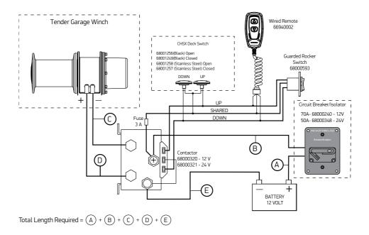
Only one type of switch is required, though more than one may be fitted.
