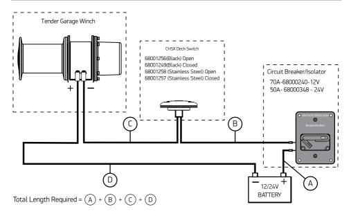
Choice of cable thickness depends on total cable length as per the following table:
